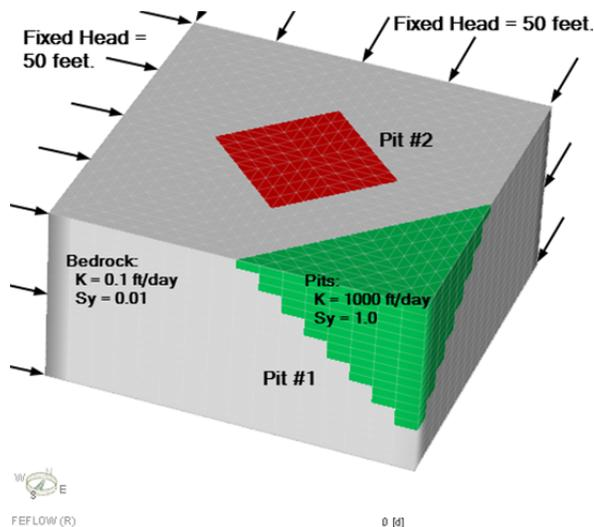
**Figure 2:** Example model configuration with mine pits.
