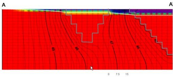
**Figure 4:** Pit-Lake results after 500 days. Head, black 0.2 ft contour lines. Water-table (zero pressure), white line.
