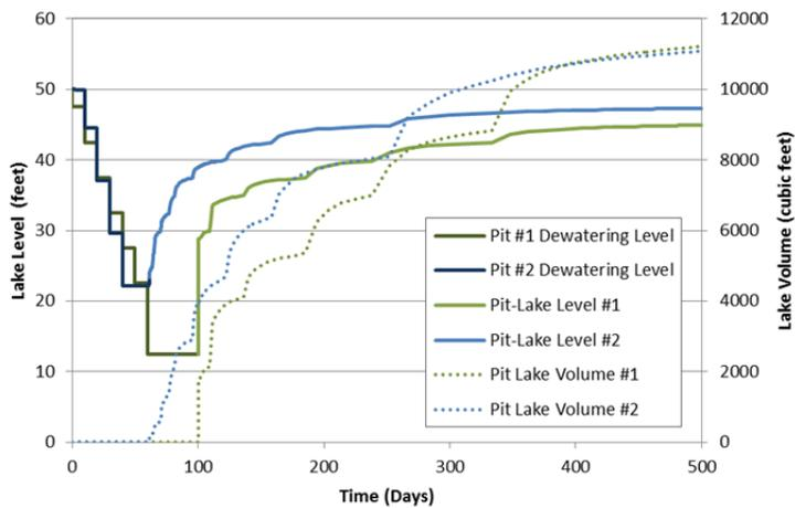
**Figure 5:** Pit level and pit-lake level and volume through time.
